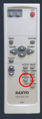
NO SHOW leaves the lamp on, but blacks out the internal display. Eventually, it will burn the display causing poor quality images and excessive heat will cause the projector to fail sooner. Power-off instead!
