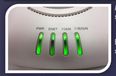
All four indicator lights on your Aruba WAPs should be green. Orange indicates a bottleneck: - ENET: The LAN connection is only 100MBit/s - 11B/G/N: The WAP is not running in N mode Backbone cabling between all Ethernet switches should be running at Gigabit speed
